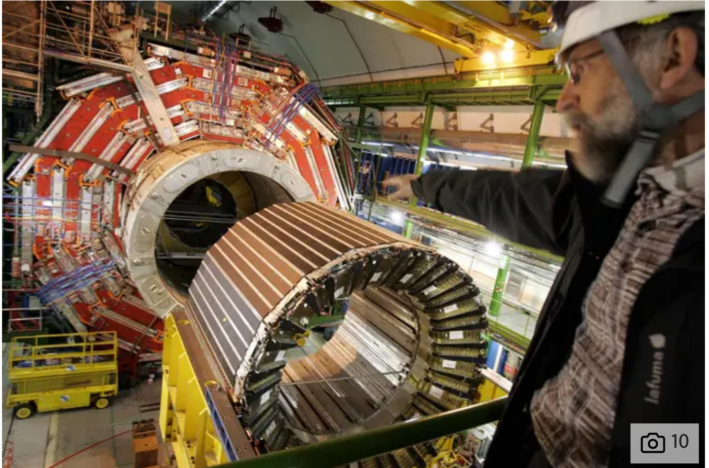
One of the world's largest superconducting solenoid magnets, part of Cern's Large Hadron Collider in Geneva (AFP/Getty)
